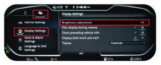
The brightness adjustment also controls the optional **DAF Corner View** Camera monitor.
