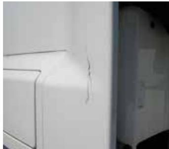
Cracks and fracture on drivers and passengers doors.
