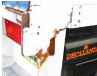
Corner of body work dented and loading edge bent.
