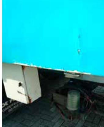
Holes or cracks in the body which are covered up with plates, filled up or refinished in a sloppy manner.
