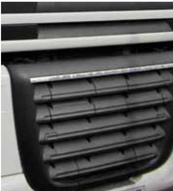
Minor damage due to stone chippings.
