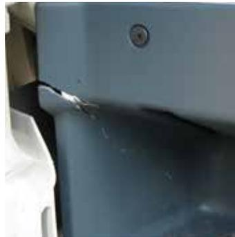
Cracks on the mudguard.
