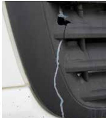
Damage and cracks on grille.
