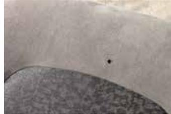
Stains on seats, which cannot be removed with a normal cleaner. Burn holes.
