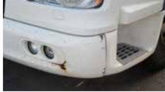
Dented, bent or deformed bumpers, excessive corrosion.
