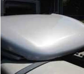
Light scratches, surface scratches on spoiler.
