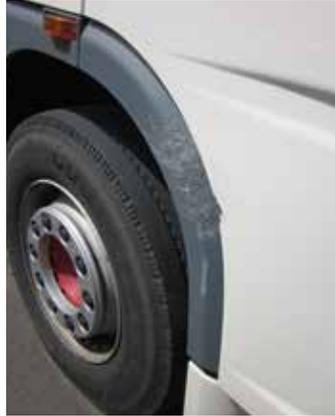
Cracks and dents caused by accident.
