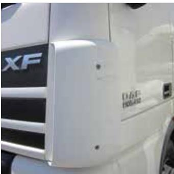
Light scratches, surface scratches on the outside of the air defectors.
