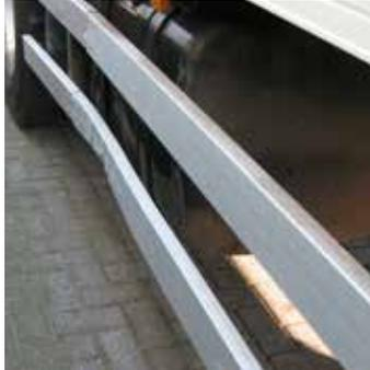
Bent or distorted under runs, including associated support.
