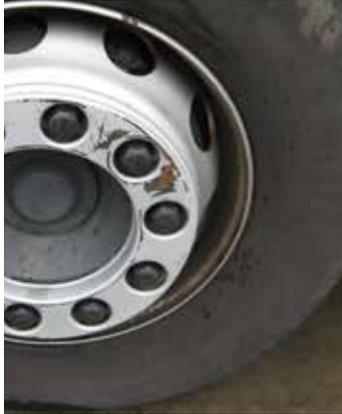
Damage to rims due to use, slight wear at the side caused by kerbs.
