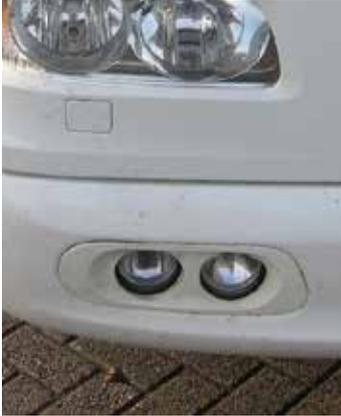
Light scratches and scrapes, which will not lead to distortions and in line with normal wear.
