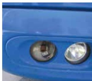
Cracks and holes in the combi-light unit.
