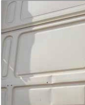
Dented back with paint damage.
