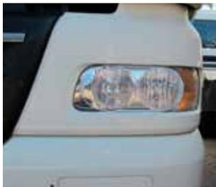
Surface scratches on lamps due to daily use. Headlamp unit is clear, no condensation and dirt is not able to penetrate.
