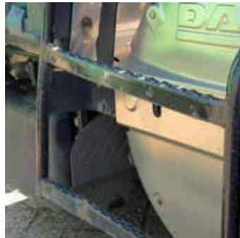
Deformed or bent stairs.
