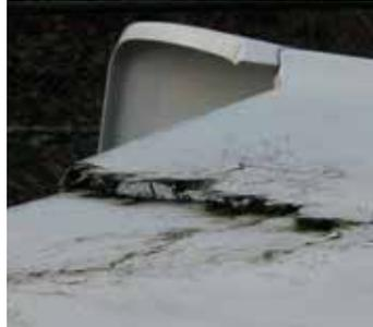
Cracks and fracture in spoiler.
