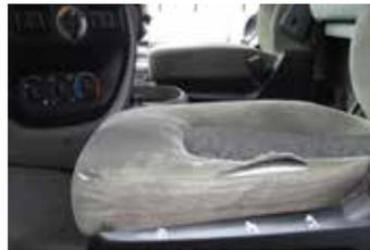
Cracks and cuts into the seat covers as a result of misuse or improper care.
