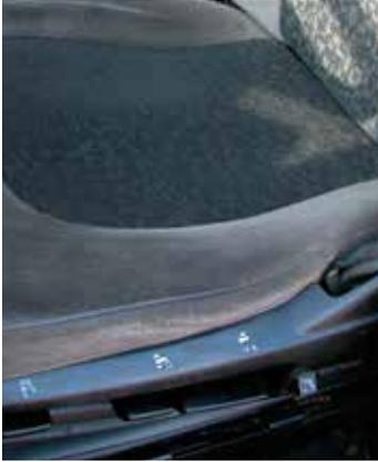
Light stains and contamination through normal use, which can be removed by regular cleaning.
