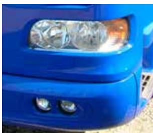
Surface scratches on the combi-light due to daily use. Combi-light unit is clear, no condensation and dirt is not able to penetrate.
