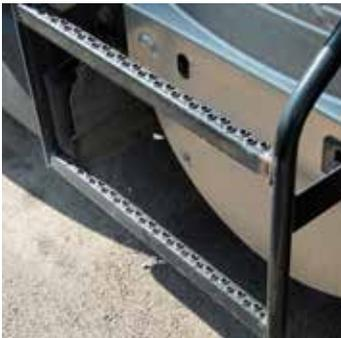
Surface scratches on stairs to catwalk.
