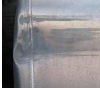
Dents in fuel tank and deformation of the fuel tank.
